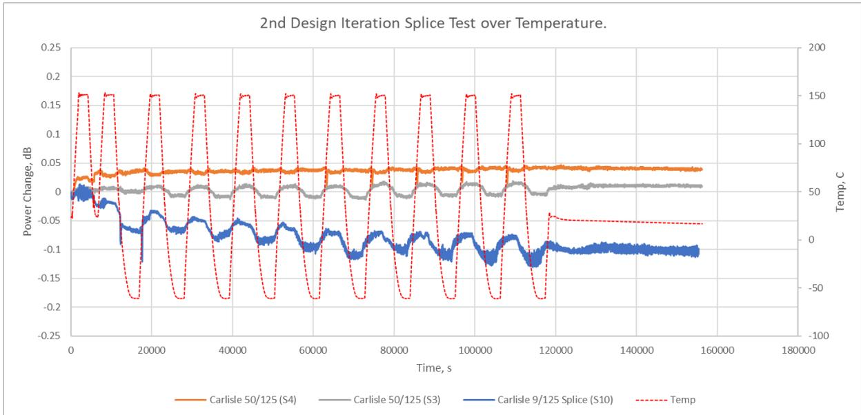
FIGURE 3 TEMPERATURE CYCLING TEST FOR 2<sup>ND</sup> DESIGN ITERATION SPLICE. EXAMPLE LOSS CHANGE DATA.
