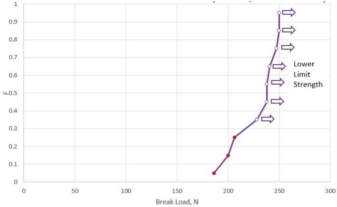
**FIGURE 9 PLOT SHOWING STRENGTH OF FERRULE CARRIER/CABLE BOND FOR 1.8 MM PFA JACKETED CABLE CURED IN AVLITECURE FIELD REPAIR OVEN. RED DATA POINTS DENOTE SAMPLE BREAKS. OPEN DATA POINTS SHOW LOWER LIMIT STRENGTH.**
